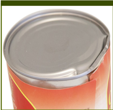
Severe dent in seam
